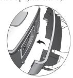
5. Turn the projector over again. Tighten the screws to hold the cable connector-panel cover and the projector on both sides.
